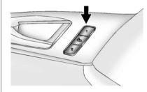
On vehicles with the memory feature, memory buttons 1 and 2 on the driver door are used to save and recall memory settings for the driver seat cushion and seatback, outside
